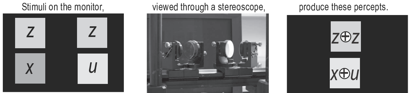
Figure 2. The first panel depicts the stimuli as displayed on the monitor. The second panel depicts the stereoscope through which respondents view the monitor. The third panel depicts the subjective percept seen by the respondents. The x, u, z are luminance values.
